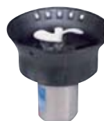
D-ICER ICE PREVENTER 78020020 Lifts the warm underwater to surface preventing the surface water from freezing. Device power: 0,75 HP/5 A 230 V, overheat protection.
