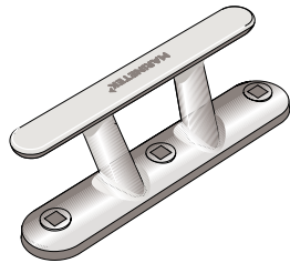
PREMIER CLEAT 62003300 Aluminium 62003340 AISI 316 Base: 88 x 444 mm Height: 135 mm Fixing: no. 3 M16 Strength: 50 kN
